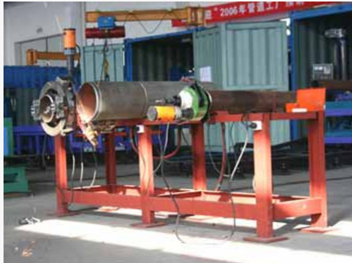
Magnetic Pipe Flame Cutting & Beveling Machine
