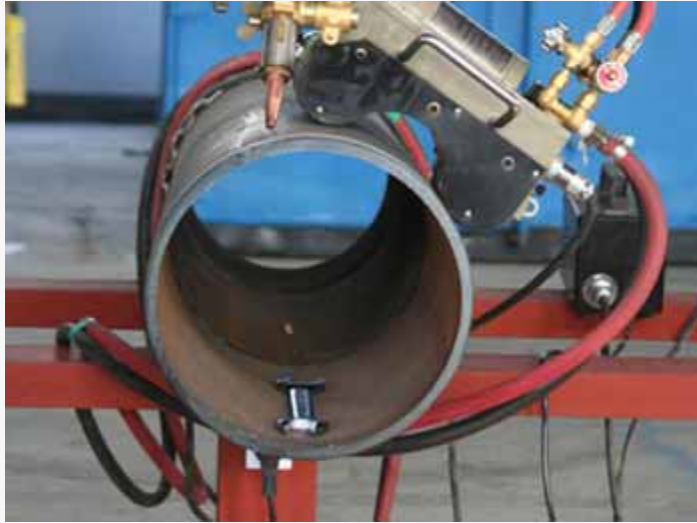
Magnetic Pipe Flame Cutting & Beveling Machine
