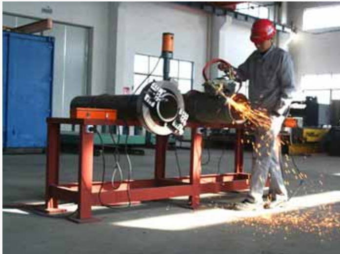
Magnetic Pipe Flame Cutting & Beveling Machine
